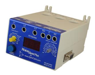
The Model 777-MV-P2 is a fully programmable electronic overload relay. It is designed to monitor and protect any 3-phase medium voltage motor drawing 10-800 full load amps. The 777-MV-P2 unit requires the use of external CTs and single-phase or 3-phase potential transformers with 100-240VAC secondaries. The unit provides unsurpassed protection from faulty voltage, underload and overload conditions. Typical applications include pumps, grinders and other 3-phase medium voltage applications.
